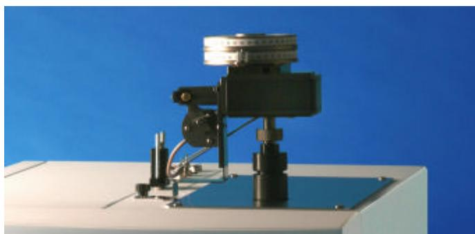
**AutoReady, Wake-up routine & Gas leak test.** The instrument allows for automatic standby at a preset time or sample position in the carousel as well as a wake-up routine at a preset time. Monitored by an intelligent electronic pressure probe, a fast and accurate fully automatic leak test procedure is available with one single key press.
